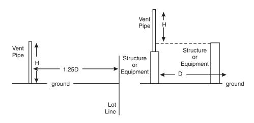
H = Minimum height in feet (mm) of vent pipe above the ground or above any structure or equipment within distance (D) where personnel might be present. D = Distance in feet (mm) to adjacent structure or equipment where personnel might be present.
